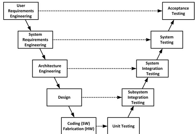
**Figure 3: System engineering “V” model (example from [6])**
